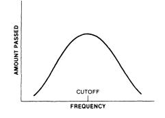
Figure 11-11. Band-pass Filter
