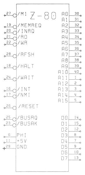
Figure 16-7. Z80 Microprocessor Pin Configuration
