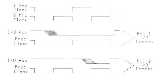
Figure 16-4. Clock Stretching in 2 MHz Mode
