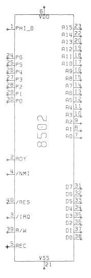
Figure 16-5. The 8502 Microprocessor Pin Configuration
