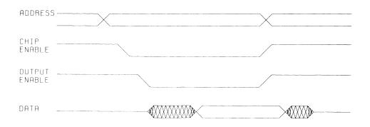
Figure 16-25. ROM Timing Diagram
