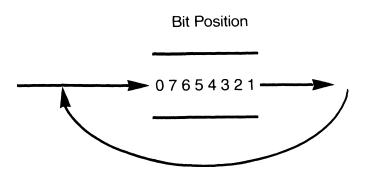
Figure 5-10. Concept of ROR (Rotate Right) Instruction
