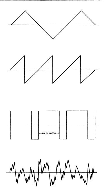
Figure 11-6. Sound Waveform Types
