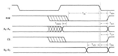
${}^{*}T_{W}$  is measured from the latest occurring of  $\phi_{2}$ ,  $\overline{CS}$ ,  $R/\overline{W}$
