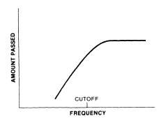
Figure 11-10. High-pass Filter
