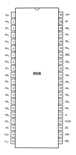
Figure 16-19. 6526 CIA Pin Configuration
