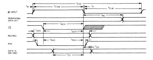
Figure 16-21. 6526 Write Timing Diagram
