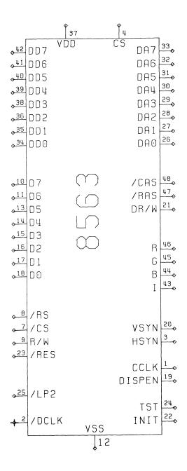
Figure 16-12. The 8563 Chip Pin Configuration
