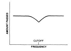
Figure 11-12. Notch Reject Filter
