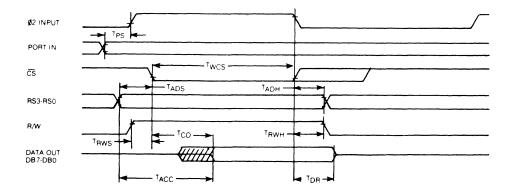
Figure 16-22. 6526 Read Timing Diagram
