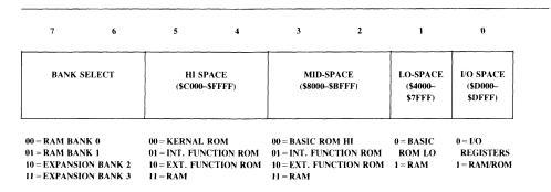
Figure 13-5. Configuration Register
