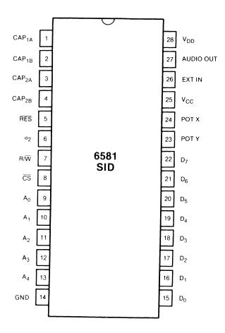
Figure 16-13. 6581 SID Pin Configuration
